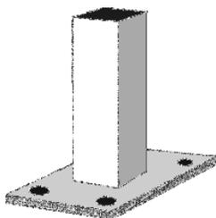
When you want to mount the fence atop your concrete pool apron, for example, you can use floor flanges on the posts. These are bolted down using lag bolts and anchors, which are available at any hardware store. You'll need four 3/8" x 2" bolts per post.
