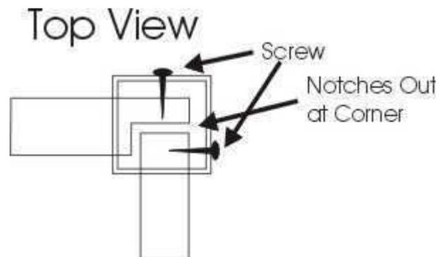
If you need to create an angle less than 90° use a corner post. It may be necessary to miter the ends of rails the closer you get to 45°; like this:
