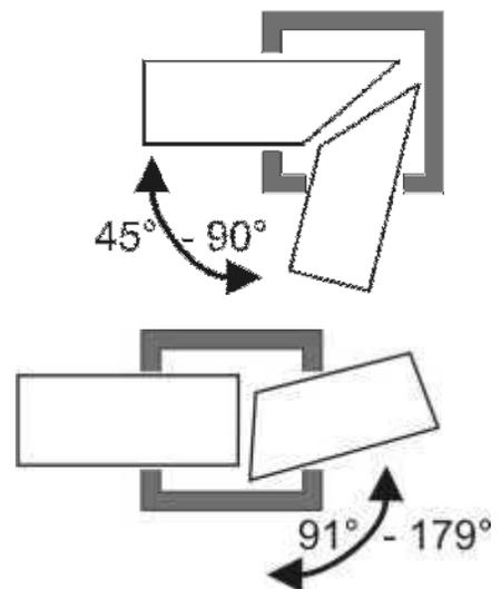
For angles greater than 90° use a line post and miter the rail ends if necessary, like this:
