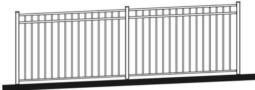
If the grade exceeds the limitations of the rackable or heavy rackable method, then a configuration as stair-stepping should be employed. The stair step method consists of blank posts and rail end brackets. The posts have no pre-punched holes, and brackets are attached to the post to hold the ends of the rails.
