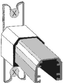
To attach fence panels to existing walls, columns or posts, you need to use rail end brackets. Brackets are screwed to the mounting surface and the rail end of the panel is inserted.
